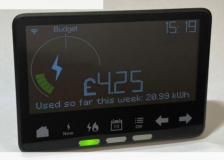
A Smart Meter is the next generation electricity meter. Smart Meters measure how much electricity you're using, as well as what it's costing you and display this on a handy in-home display. In the future these will allow us to better understand our network through data gained from Smart Meters.
