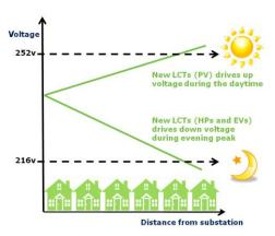
switches, on-load tap changing transformers and monitoring devices that communicate with our network management system. The closed loop control system operates to ensure that there are no network voltage violations and reconfigures the network to optimise for power flow and losses.
