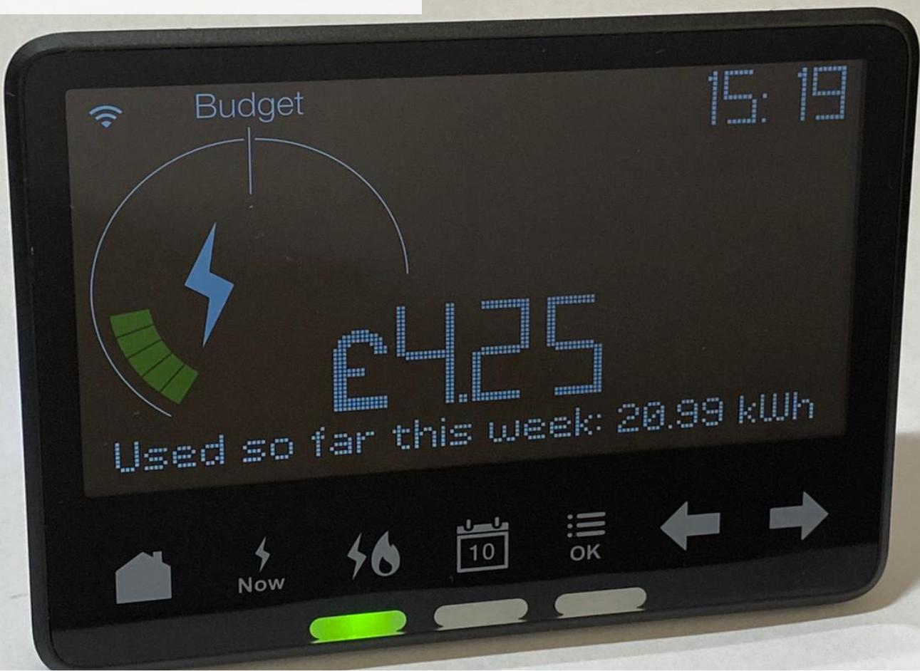
A Smart Meter is the next generation electricity meter. Smart Meters measure how much electricity you're using, as well as what it's costing you and display this on a handy in-home display. In the future these will allow us to better understand our network through data gained from Smart Meters.
