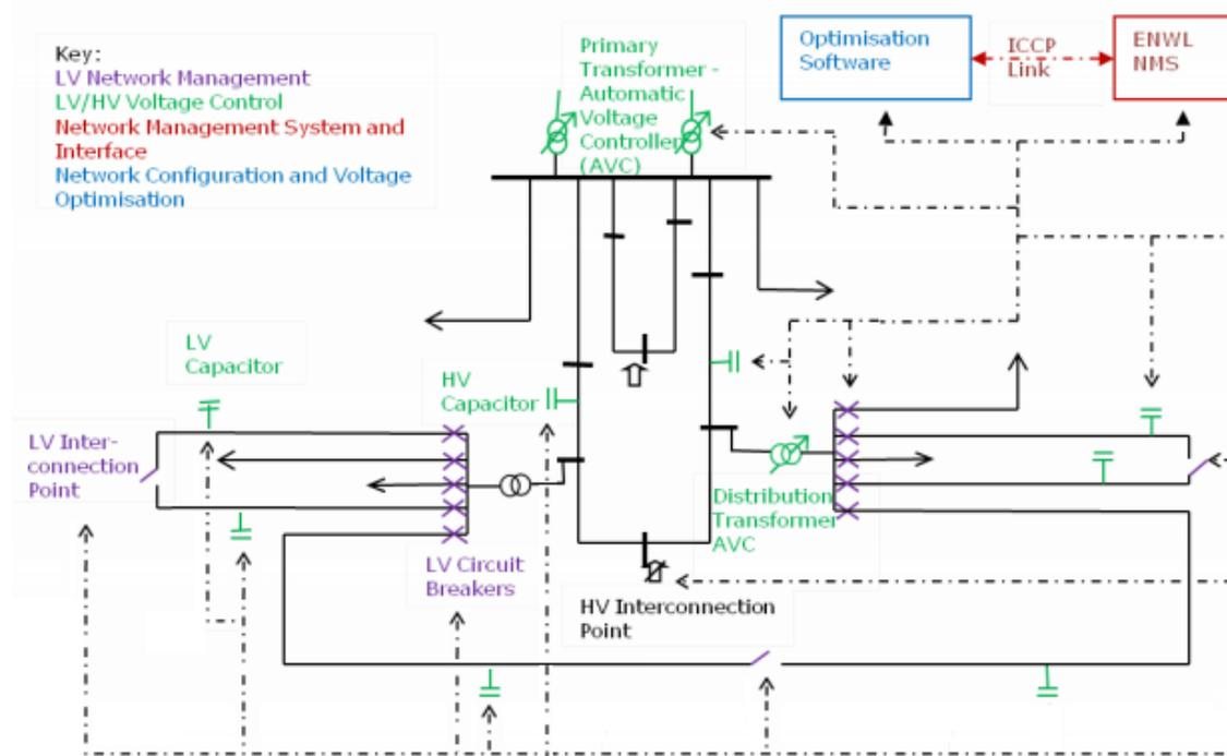
The LV network control will be established using new retrofit LV vacuum circuit breaker, WEEZAP and retrofit remote control link box switch, LYNX. Deploying the WEEZAP in conjunction with the LYNX will allow LV network interconnection and facilitate dynamic reconfiguration either locally or remotely from Electricity North West's Control Room. Where a link box does not exist at a proposed interconnection point then a new link box will be installed to allow the reconfiguration capability.
