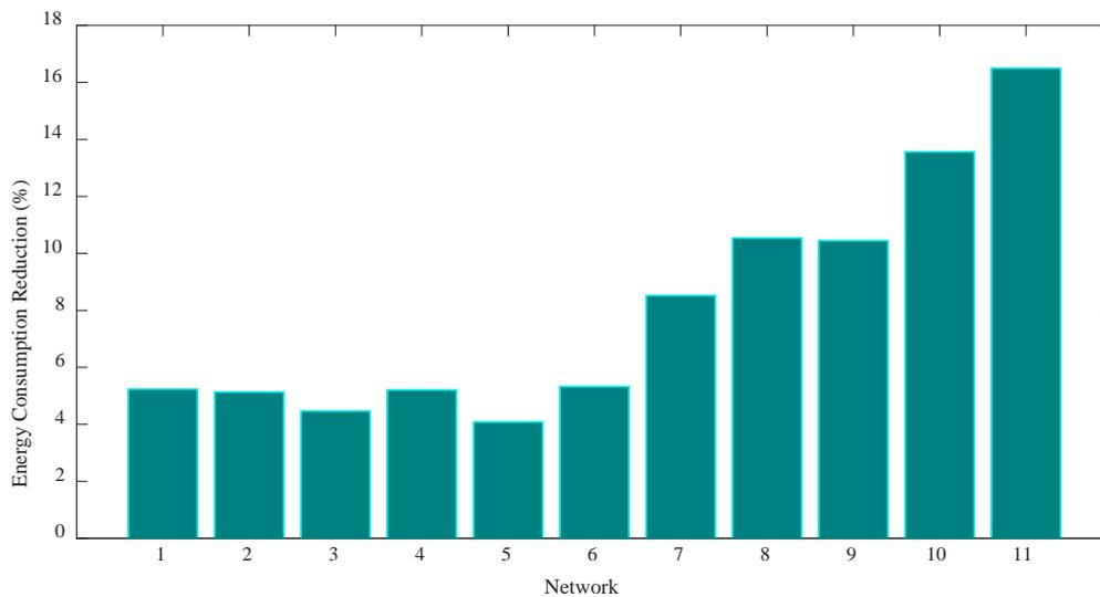
Figure 7: Percentage reduction in LV network energy losses
