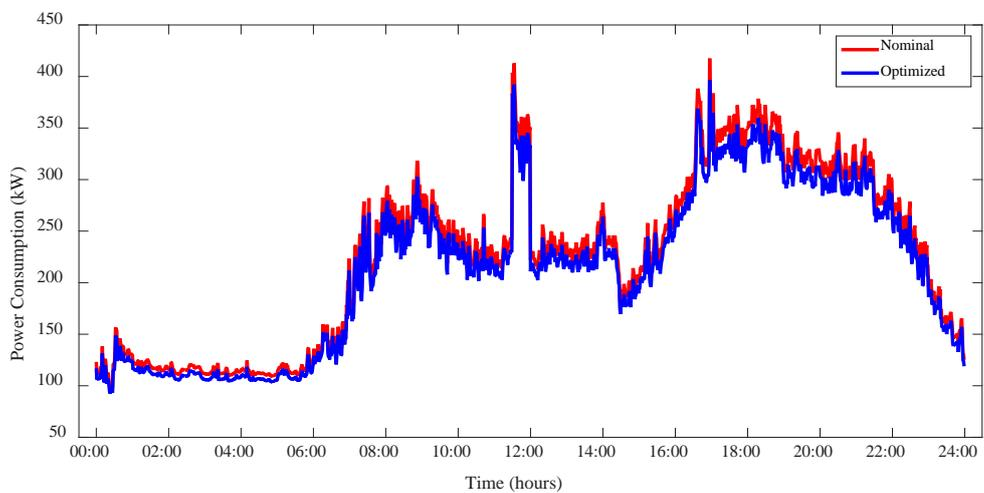
Figure 14: Power consumption network 9 with OLTC
