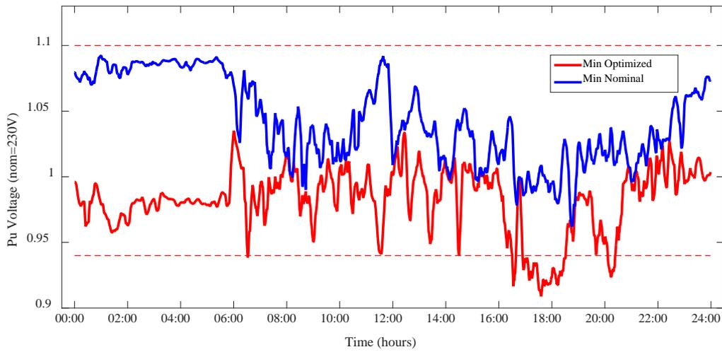
Figure 16 : CVR tap settings network 3 with an OLTC
