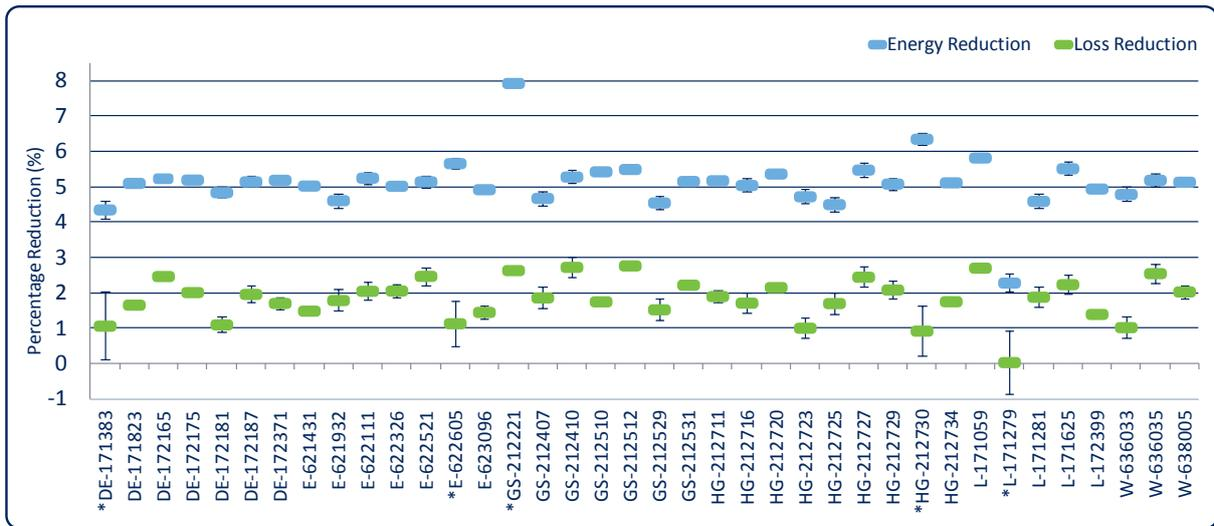
Figure 5: Energy and loss reduction on HV networks using CVR model
