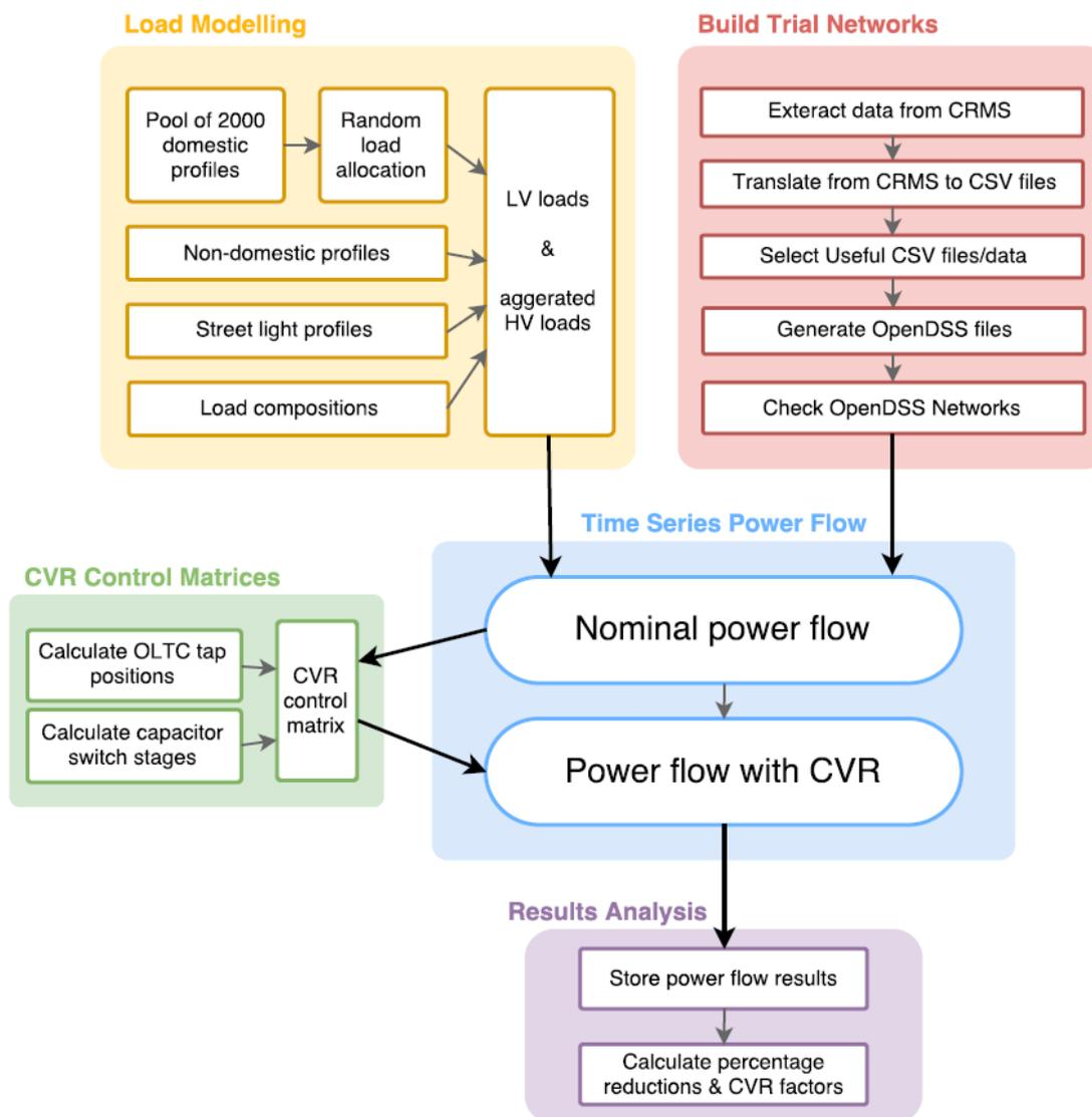
The simulation results from the nominal power flow are used to calculate the CVR control matrices – one for the HV network and one for the LV network.
