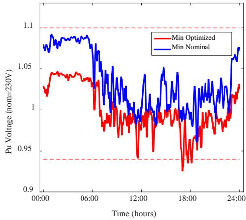
Figure 9: Voltage profile network 9 with OTLC
