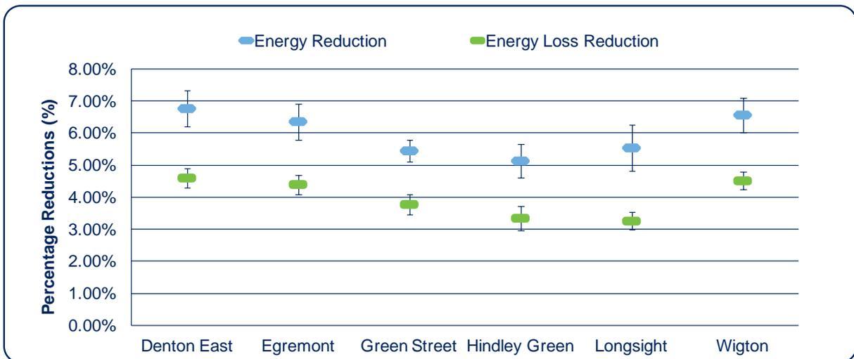
According to the simulation results the CVR model is capable of providing energy and loss savings to all LV and HV networks.
