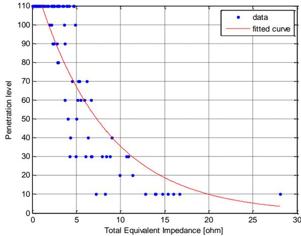
**Figure 70: Total Path Impedance,  $R^2:0.78$  – EHP Case**
