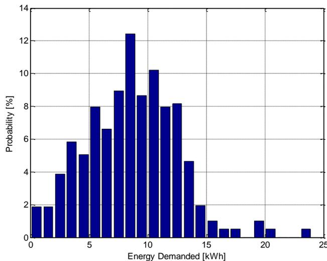
**Figure 10: Probability distribution function for the daily EV energy requirement**
