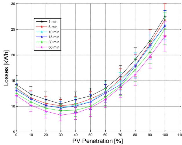
Figure 39: Daily energy losses – Data granularity
