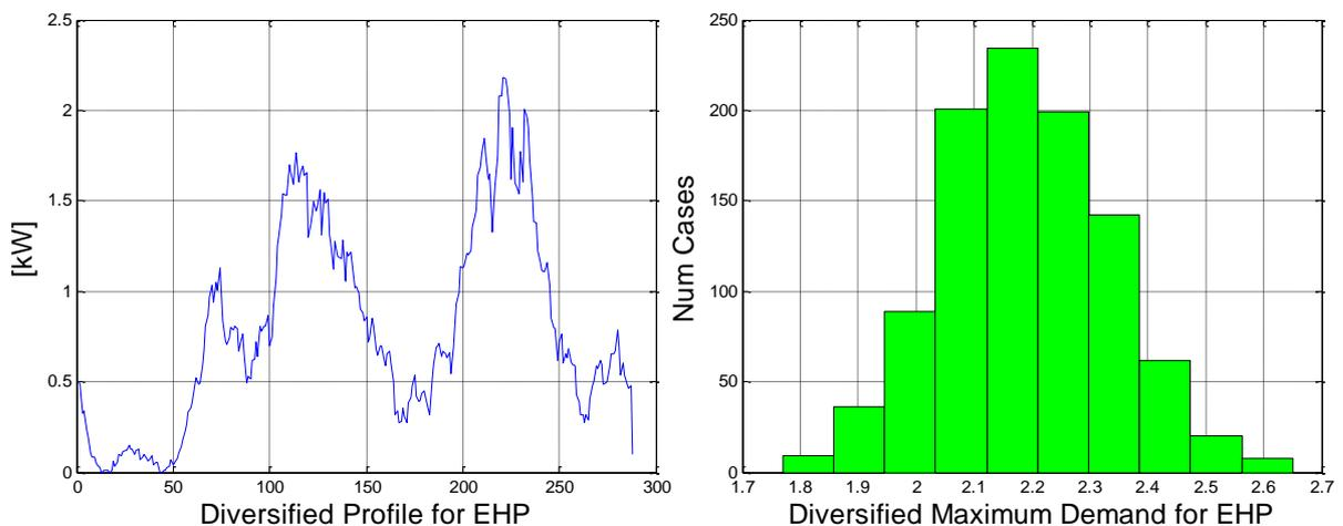
**Figure 15: Diversified Profile and Maximum Demand Histogram for 100 EHP profiles**
