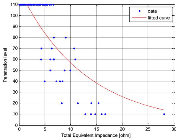
Figure 73: Total Path Impedance,  $R^2:0.70$  – EV Base Case
