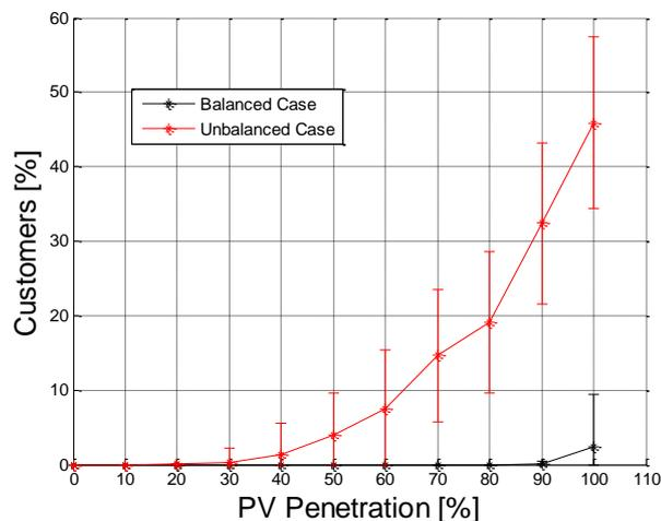
Figure 36: Percentage of Customers with Voltage Problems – Comparison
