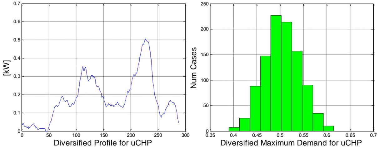
**Figure 16: Diversified Profile and Maximum Demand Histogram for 100 μCHP profiles**
