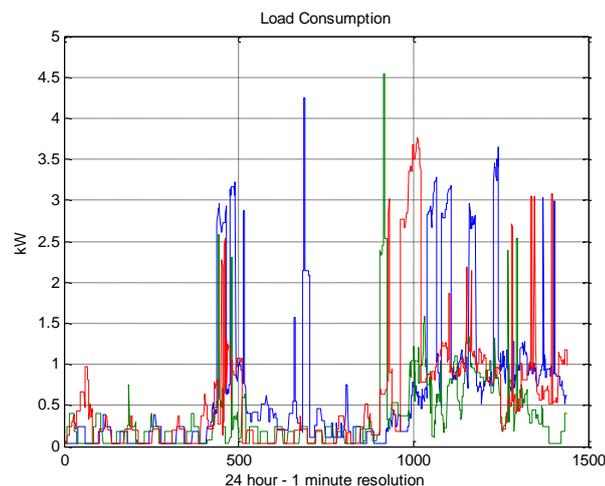
Figure 1: Individual load profiles – 1 minute resolution
