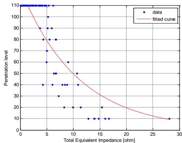
Figure 79: Total Path Impedance,  $R^2:0.75$  – EV Shifted Case
