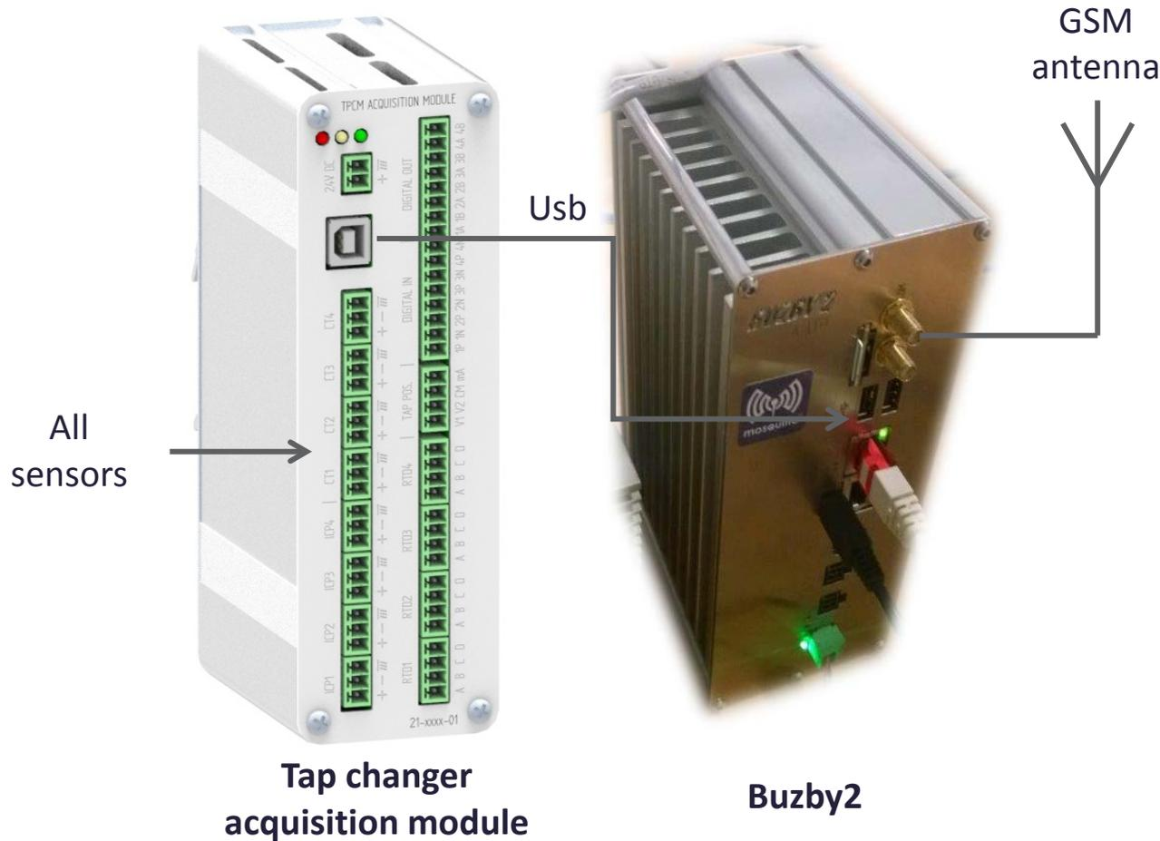
Complete custom USB acquisition module designed
