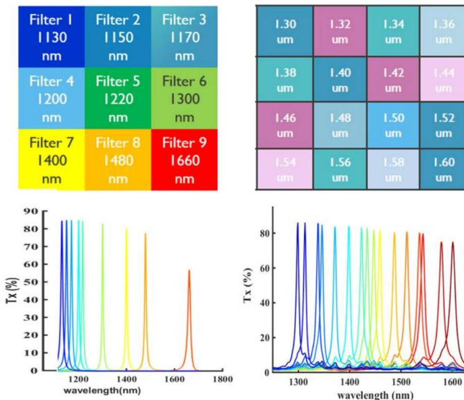
Figure 7: Arrangement of filters in 9-band (top left) and 16-band (top right) Snapshot SWIR detectors, and transmittance of each (bottom left and bottom right). From imec [20].
