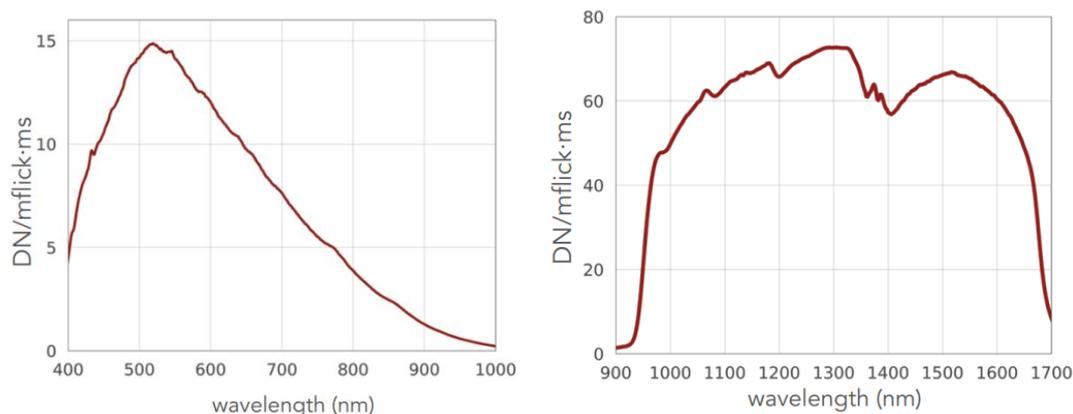
Figure 10: Spectral response curves for Resonon Pika XC2 (left) and Pika IR+ (right). From [22] and [24].
