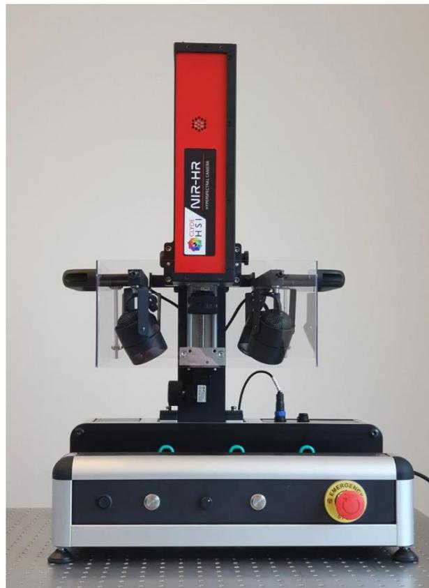
Figure 3: Transportable scanning system consisting of NIR-HR camera, two lights, and conveyor stage, from ClydeHSI [11].
