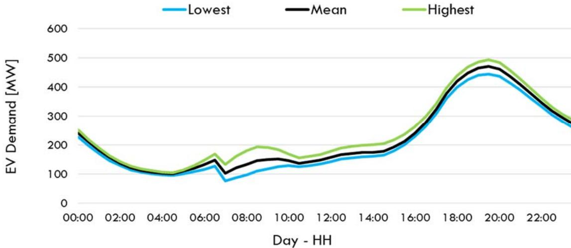
**Fig. 1. Aggregated EV charging demand profile across all BSPs for a typical winter day in FY28. Results shown for the lowest, mean and highest EV charging demand profiles taking into account all 50 micro-scenarios.**
