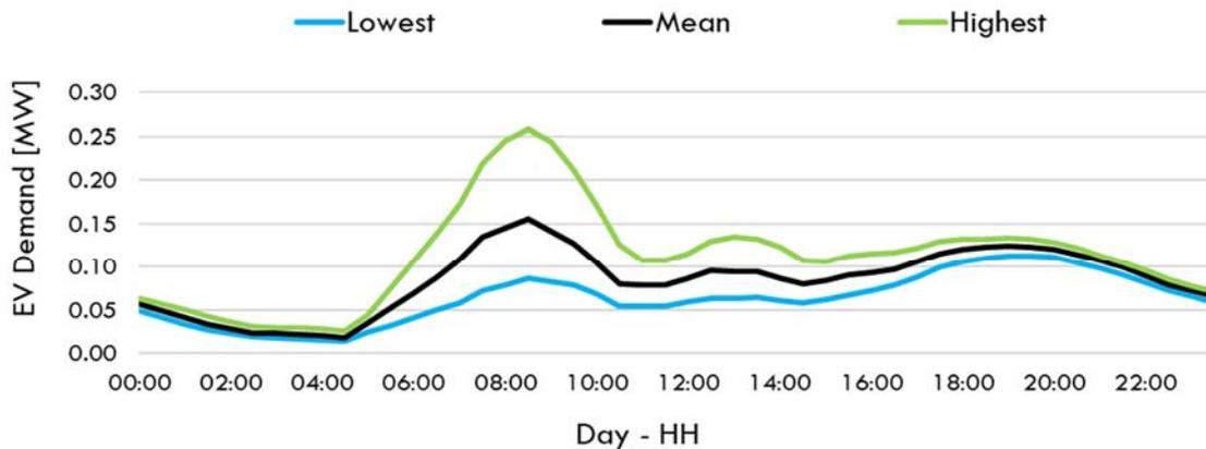
**Fig. 4. EV charging demand profiles for Manchester University primary substation for a typical winter day in FY28. Results shown for the lowest, mean and highest EV charging demand profiles taking into account all 50 micro-scenarios.**
