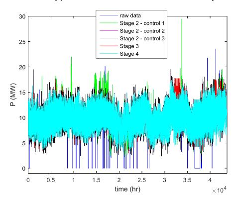
Fig. 7. Half-hourly processed P demand data of BSP#7 of Electricity North West Ltd.
