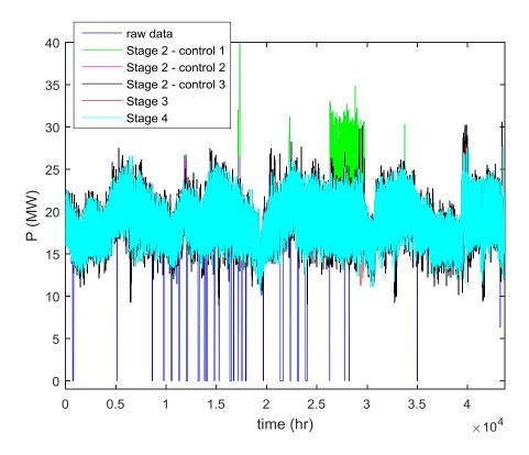
Fig. 8. Half-hourly processed P demand data of BSP#8 of Electricity North West Ltd.
