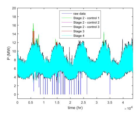
Fig. 14. Half-hourly processed P demand data of primary substation #4 of Electricity North West Ltd.
