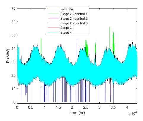
Fig. 6. Half-hourly processed P demand data of BSP#6 of Electricity North West Ltd.
