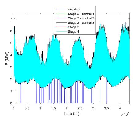
Fig. 11. Half-hourly processed P demand data of primary substation #1 of Electricity North West Ltd.
