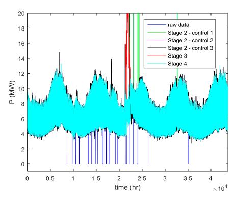
Fig. 15. Half-hourly processed P demand data of primary substation #5 of Electricity North West Ltd.
