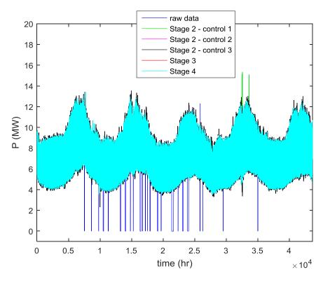
Fig. 19. Half-hourly processed P demand data of primary substation #9 of Electricity North West Ltd.
