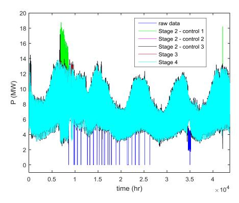
Fig. 20. Half-hourly processed P demand data of primary substation #10 of Electricity North West Ltd.
