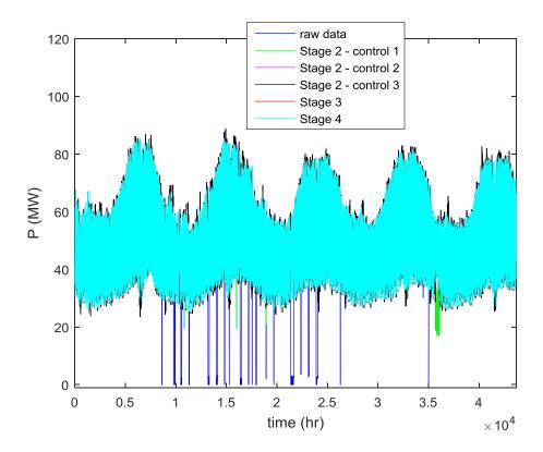
Fig. 1. Half-hourly processed P demand data of BSP#1 of Electricity North West Ltd.
