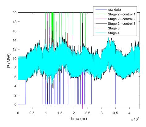
Fig. 18. Half-hourly processed P demand data of primary substation #8 of Electricity North West Ltd.
