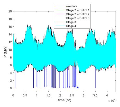
Fig. 17. Half-hourly processed P demand data of primary substation #7 of Electricity North West Ltd.
