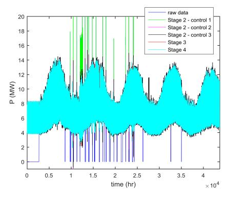
Fig. 12. Half-hourly processed P demand data of primary substation #2 of Electricity North West Ltd.
