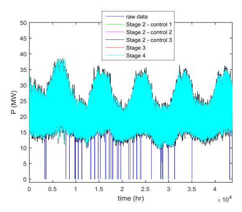
Fig. 10. Half-hourly processed P demand data of BSP#10 of Electricity North West Ltd.
