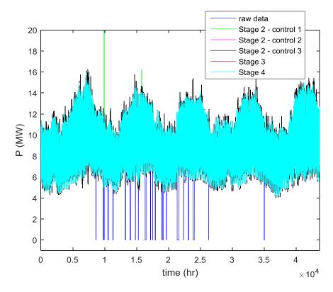
Fig. 16. Half-hourly processed P demand data of primary substation #6 of Electricity North West Ltd.
