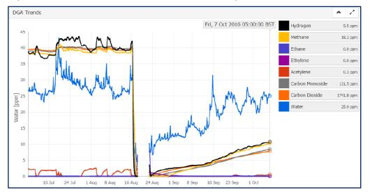
Figure 5.5: Chemical trends before and after oil regeneration – Barton Dock transformer
