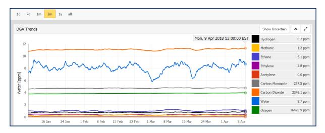
Figure 5.7: Successful oil regeneration – Peel substation, April 2018
