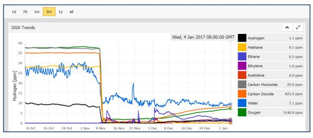
Figure 5.6: Successful oil regeneration – Peel substation, January 2017
