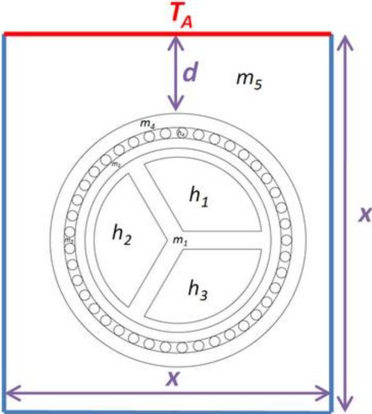
The drawing is then imported into the software package and each of its objects is allocated the material properties of the component that they represent.
