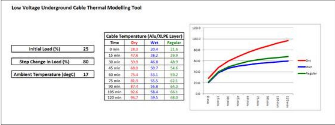
The methodology used to develop this tool can be extended to other cable types and/or feeder arrangements in the future. Additionally, LV-TM can be extended to other time-varying load and ambient temperature profiles as well as different types of soil and levels of soil moisture content.
