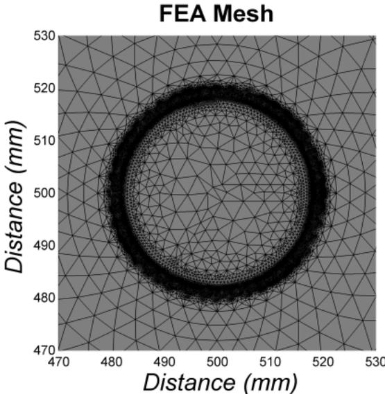
An electrical model was used to determine the phase current profiles to be used as inputs to the thermal model in order to calculate temporal variation of temperature in the cable.
