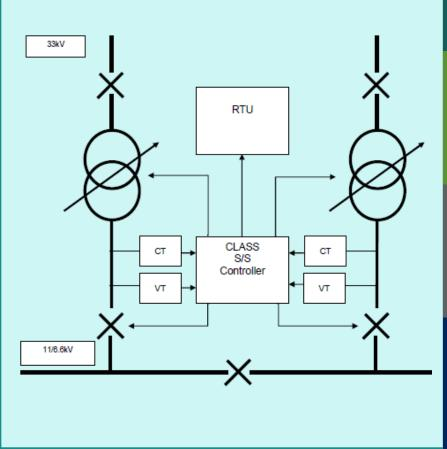
Primary Frequency Response LV circuit breaker opens when frequency falls below a set threshold
