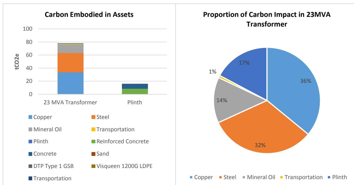
Figure 2 Asset Carbon Impact embodied in transformers
