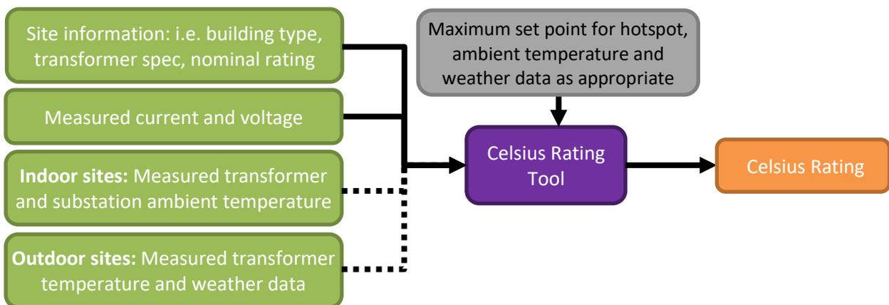
Figure 4: Functionality of the Celsius Rating Tool
