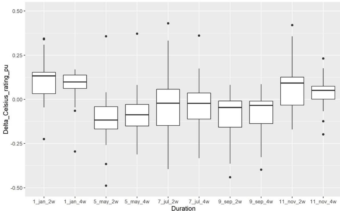
**Figure 5: Comparison of Celsius rating calculated from 2 and 4 weeks' worth of data and the baseline data which was for more than 3 years**
