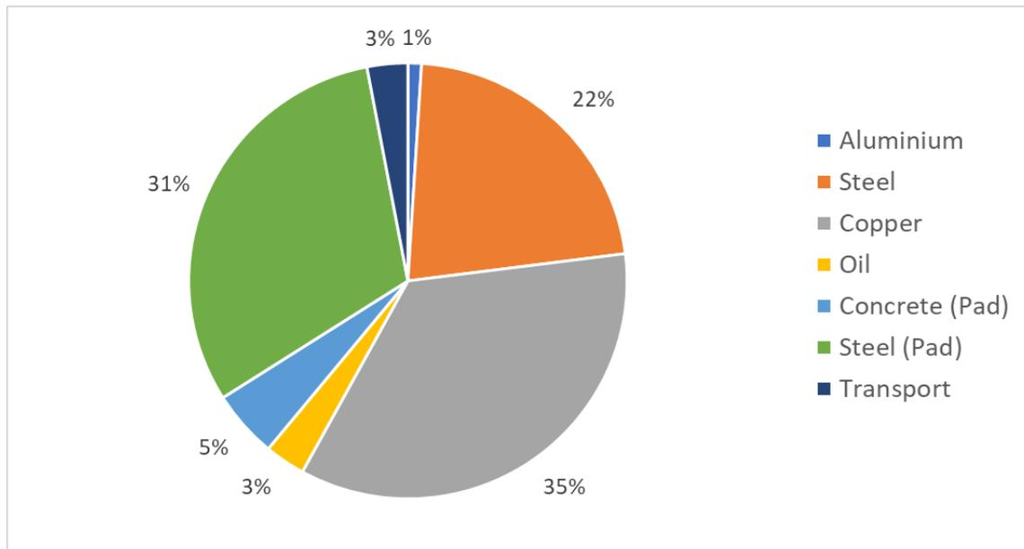
**Figure 2:** Materials and their proportions used in assessing carbon impact of transformers
