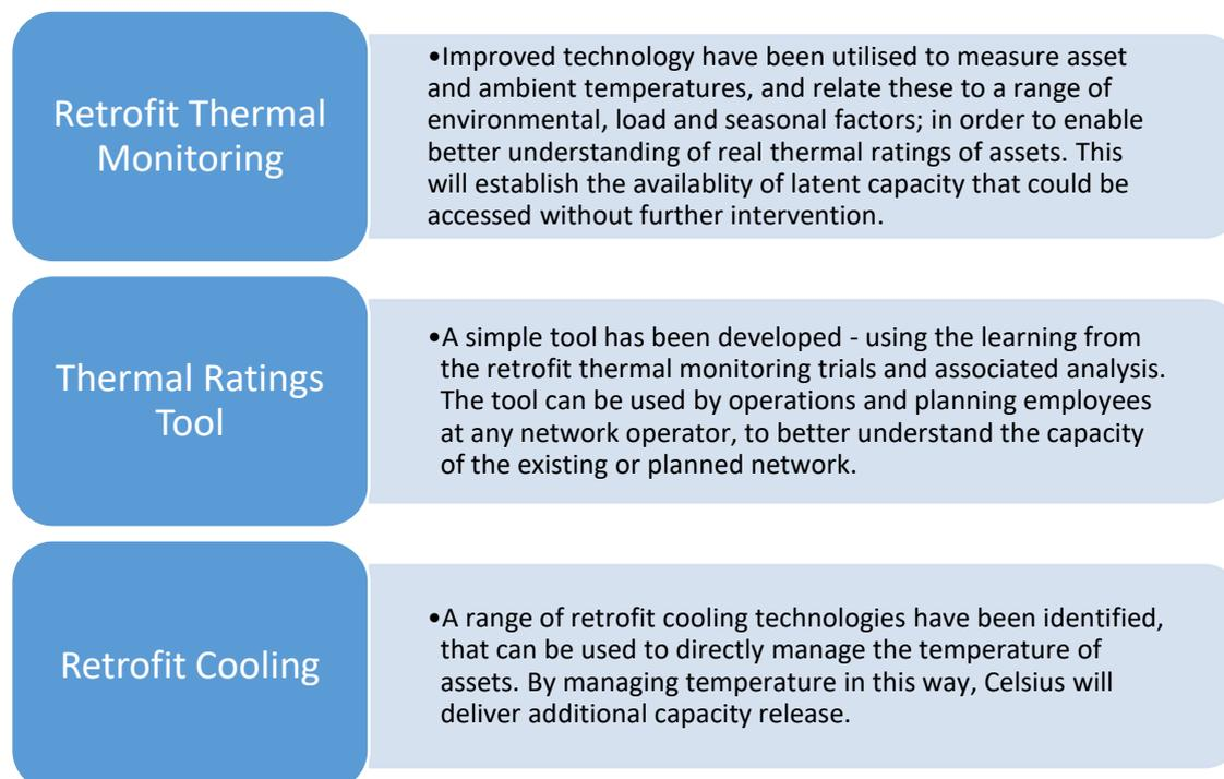
**Figure 1:** Celsius methodologies for thermal management at electricity substations
