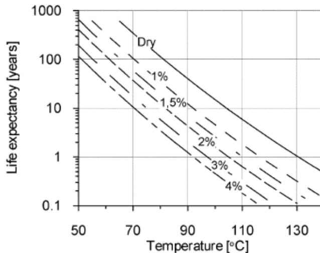
**Figure 4 - Expected life for solid insulation and its dependence upon moisture and temperature, as reported by Lundgaard [6]**
