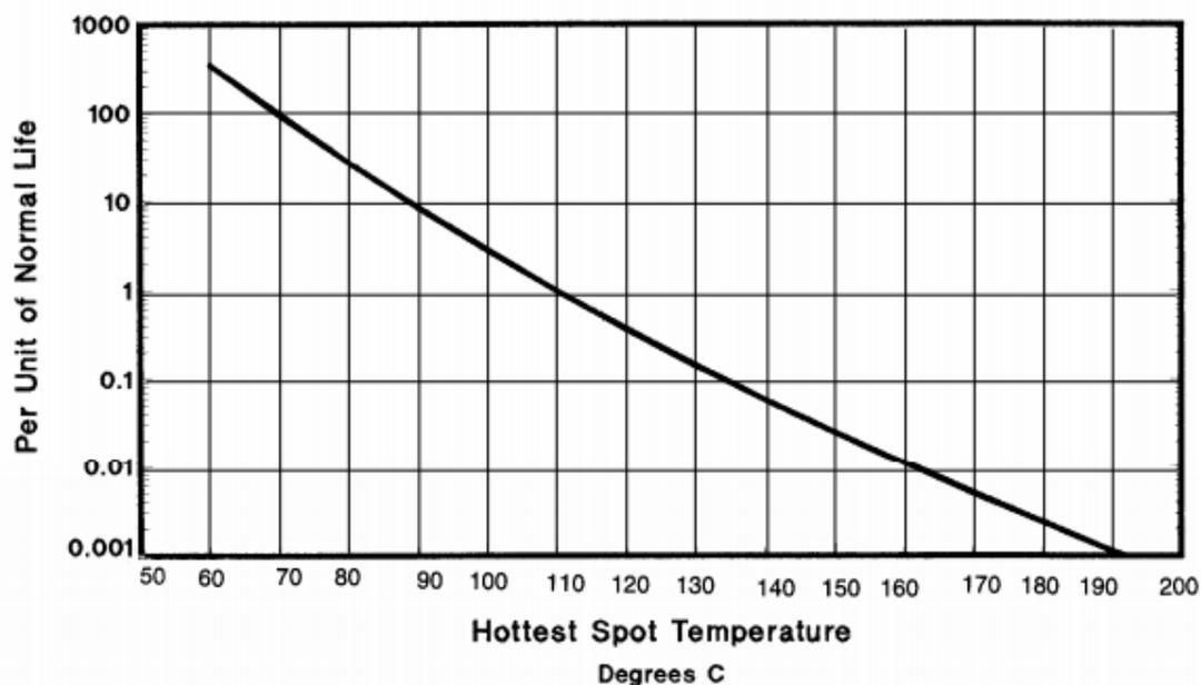
**Figure 7 - IEEE C57.91 transformer insulation life curve, normalised to 110°C hot spot temperature (noting that this yields 20.5 years life according to IEEE C57.91)**
