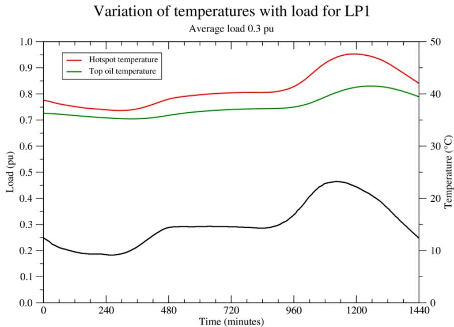
**Figure 10 – Variation of hotspot and top oil temperature with load for LP1 with 30% average utilisation at 20°C ambient**
