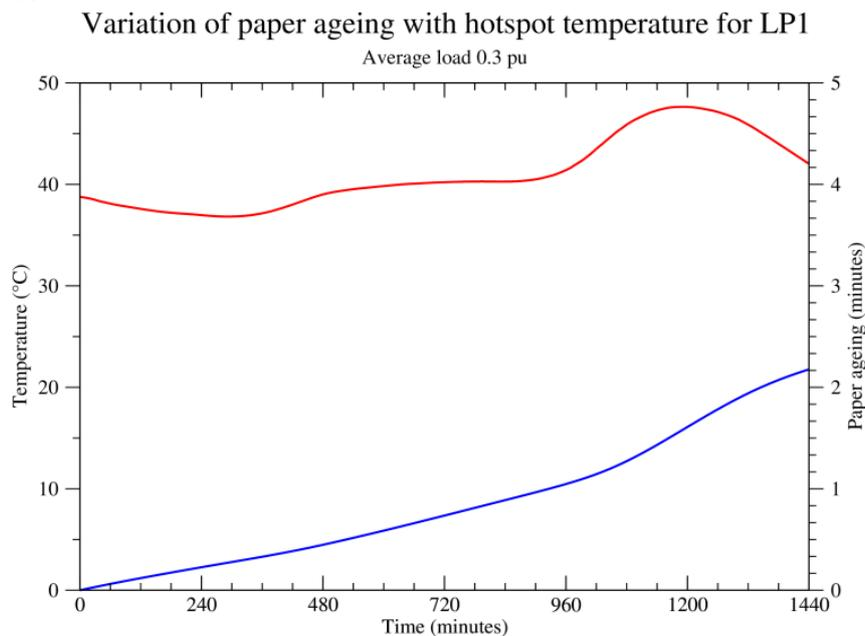
**Figure 11 – Variation of hotspot temperature and insulation ageing with load for LP1 with 30% average utilisation at 20°C ambient**
