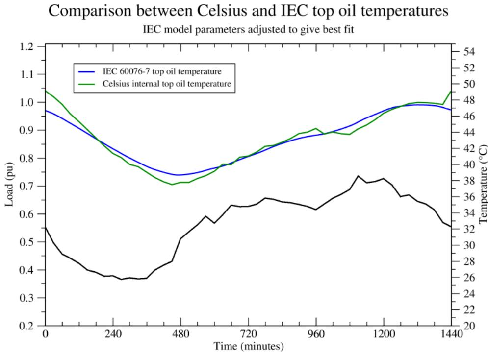
**Figure 14 – Top oil temperature calculated from Ricardo equations compared with possible fit from IEC 60076-7 model for example given in Daily Rating tool**
