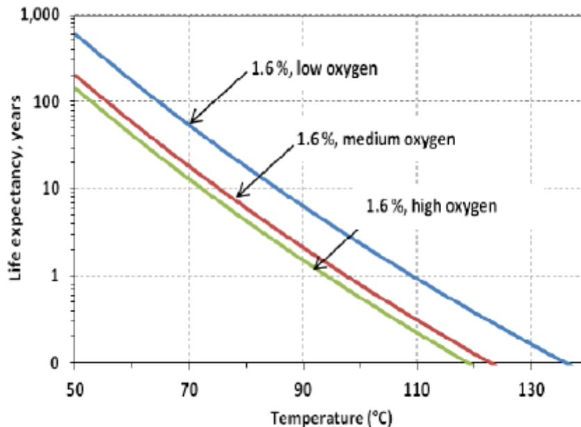
**Figure 6 – Life curves for Kraft paper with 1.6% water in different oxygen environments, reproduced from [11]**
