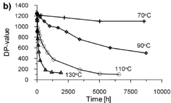
**Figure 3 - DP versus ageing time for paper with 3% moisture added [6]**
