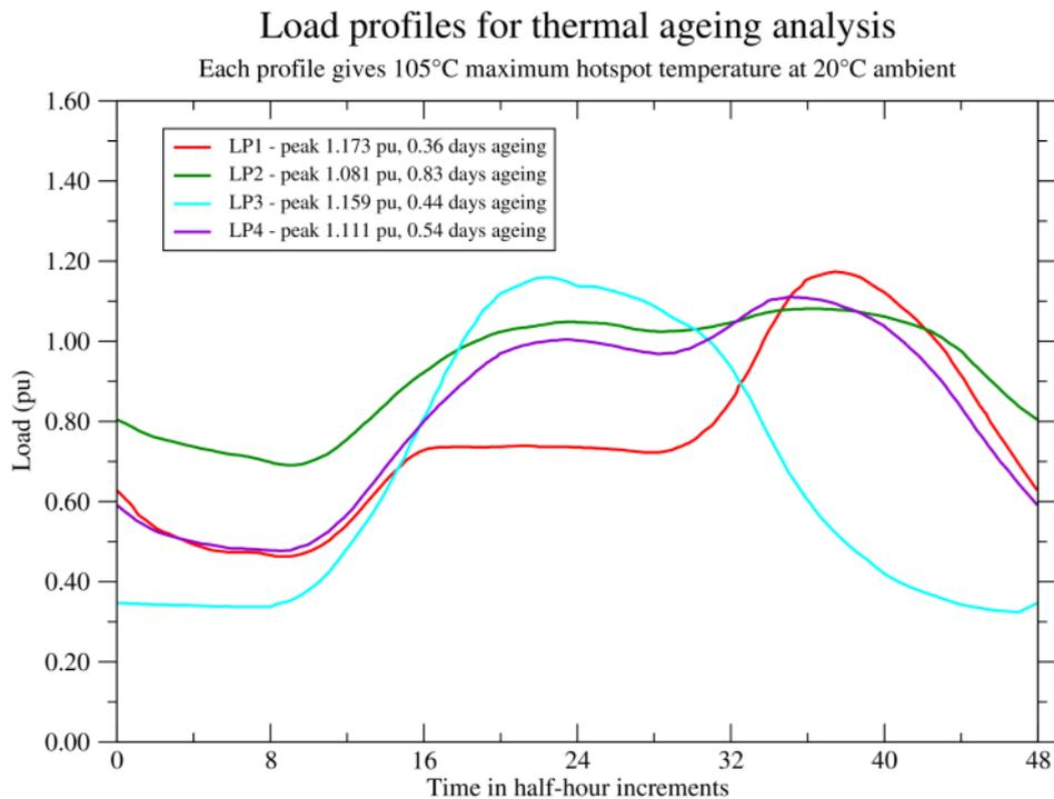
**Figure 13 – Load profiles for thermal ageing analysis with each curve scaled to give a maximum hotspot temperature of 105°C at 20°C ambient**
