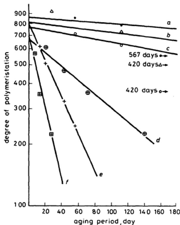
**Fig. 6** Effect of water on the rate of aging under nitrogen at 120°C
