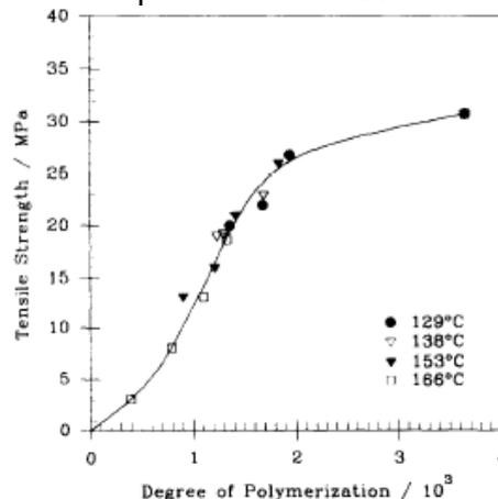
**Figure 2 - Relationship between tensile strength and degree of polymerisation for artificially aged paper, reproduced from [7]**
