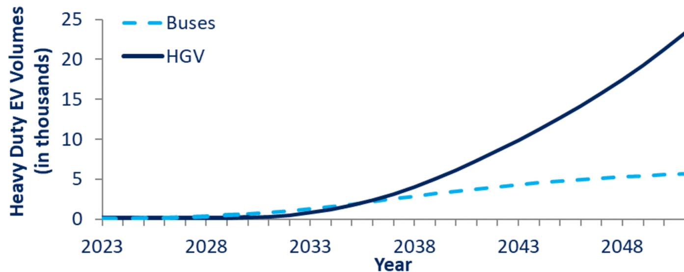
Electrification is expected to be the main path to decarbonise the transport sector, especially for light duty vehicles such as cars and vans. It is also anticipated that a notable proportion of heavy-duty vehicles, particularly buses and trucks under 25 tonnes, will be electric and will predominantly rely on electricity distribution networks for their battery charging.
