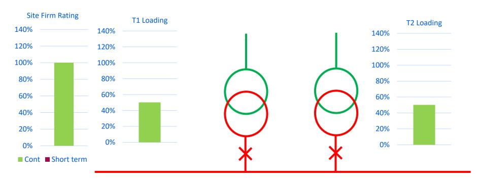
• 100% of the total substation load can be shared, so 50% loading on each transformer
