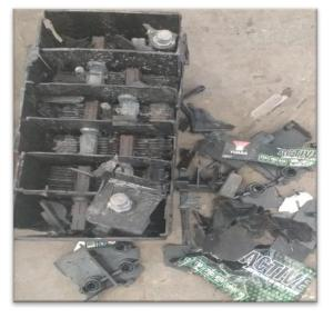
To prevent further incidents, users must ensure vehicle batteries are not overloaded.
