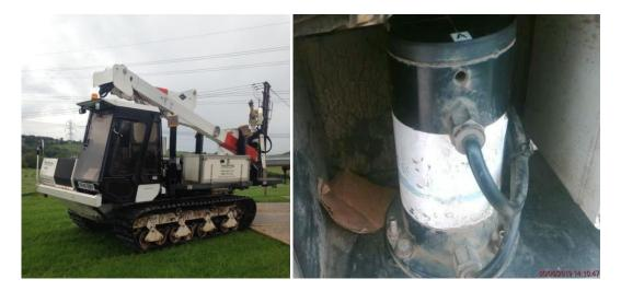
An inspector discovered that the tilt sensor, a critical safety device fitted to prevent overturning during extension of the boom, appeared to have been tampered with in an apparent attempt to override the safety function.
