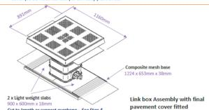
The depth from the top of the composite mesh base to the pavement level shall be 710mm maximum and 640mm minimum
