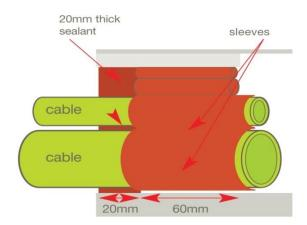
Once the installation of the Nofirno Duct Seal system is complete a 6 point check should be made on each installation.
