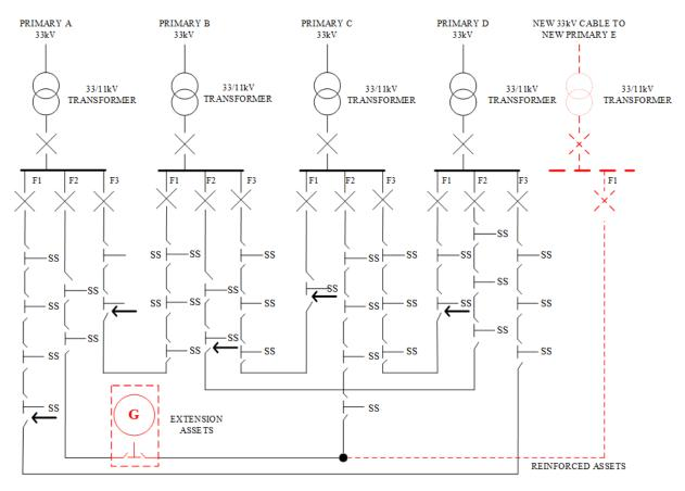
The existing network consists of four 10MVA primary transformer substations and associated 11kV switchgear. A new connection of 4MVA has been requested in the vicinity of F2 from Primary A.
