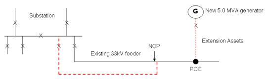
Reinforcement Assets : New 33kV feeder 24.0 MVA Thermal Capacity
