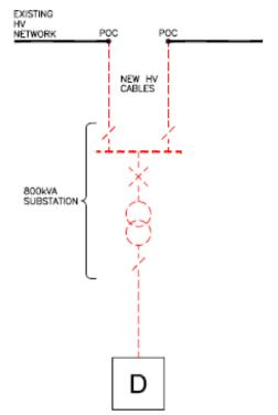
b) The Minimum Scheme is as for scenario a) above but the Customer requests an enhanced connection arrangement where the substation is looped into existing HV network.
