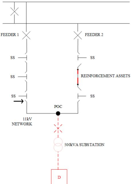
The Relevant Section of Network is the two-feeder ring comprising Feeder 1 and Feeder 2. As this is a Demand Connection, no CAF contribution is required. The High-Cost Project Threshold (HCPT) applied is the Required Capacity x HCPT of  $\pounds$ 1,720 per kVA.
