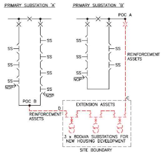
The assets connecting POC A and POC B add capacity to the existing network, so would normally be treated as Reinforcement. These comprise –
