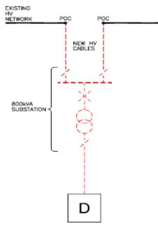
b) The Minimum Scheme is as for scenario a) above but the Customer requests an enhanced connection arrangement where the substation is looped into existing HV network.
