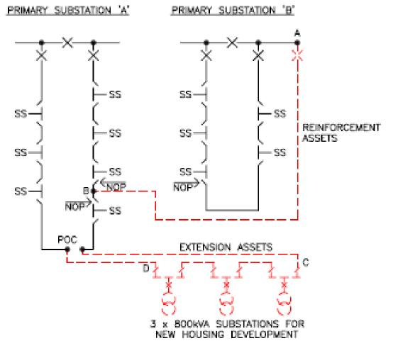
The figure below shows the proposed Reinforcement and POC to the 11kV network:
