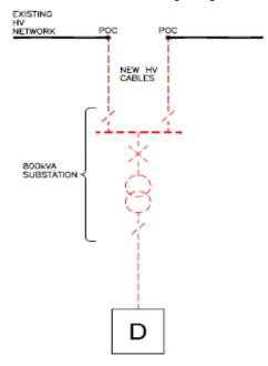
b) The Minimum Scheme is as for scenario a) above but the Customer requests an enhanced connection arrangement where the substation is looped into existing HV network.
