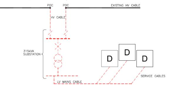
The Connection Charge for this Scheme is calculated as follows:
