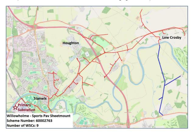
Currently two of the four normally open points on this circuit are not automated. This is impacting restoration performance, especially the backfeed at Whoof House which is the main alternate supply to the WSC section. It is proposed that all NOPs on this circuit are fitted with remote control to improve automation performance.
