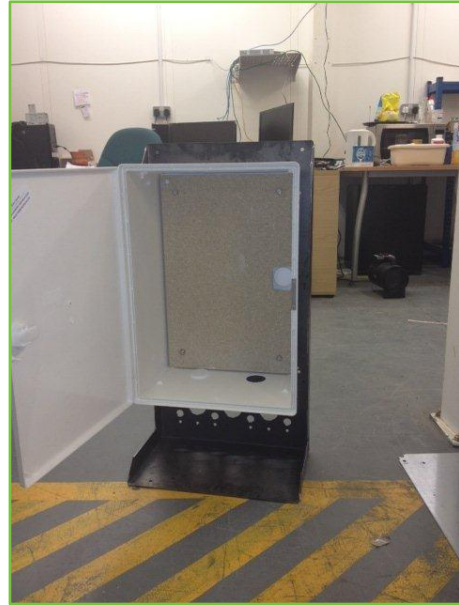
Figure 4 – Electrotech Mounting Frame for Outdoor Installation, plus Cabinet for GridKey Monitoring Unit
